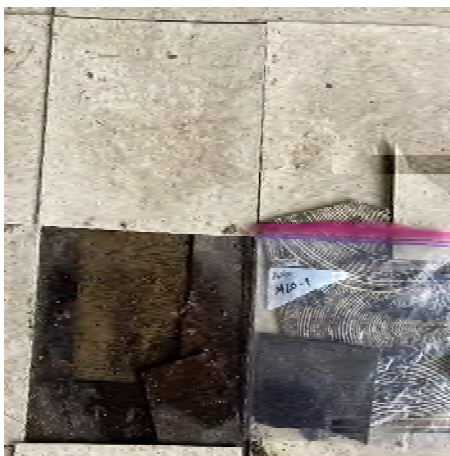
Photo 7 Black floor tile (6% Chrysotile) and adhesive (6% Chrysotile)
